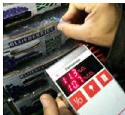
Fig. 2: Measuring gas compositions upon arrival in China.
